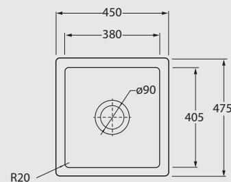
**PLEASE NOTE:** A DXF is not available, sink should be used as template. When undermounting, a minimum gap of 4mm must be left between the sink and the worktop.
