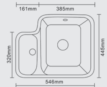
**PLEASE NOTE:** A DXF is not available, sink should be used as template. When installing, a minimum gap of 4mm must be left between the sink and the worktop.
