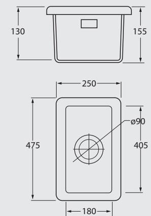
**PLEASE NOTE:** A DXF is not available, sink should be used as template. When undermounting, a minimum gap of 4mm must be left between the sink and the worktop.
